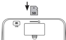
2. To remove the SD card, press it in until it clicks and pops out, then remove it from the SD card slot.
