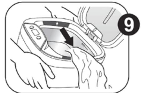
**Note:** To avoid residue building up, always empty the tank and wipe it clean. Recommend using fresh water each time.
