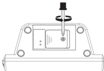
2. Remove the battery compartment panel
