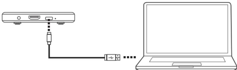
1.1 - Connect the Micro USB cable to the power input on the back of the PP60 and connect the USB end to a computer or USB power adapter.
