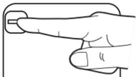
Lightly turn the focus wheel on the projector to fine-tune/ focus the picture.
